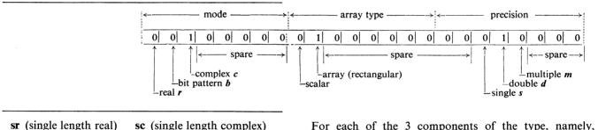
For each of the 3 components of the type, namely, precision, mode, and array type there are 8 possibilities, some of which are spare. The full type of an operand is therefore given by a single bit in each of the 3 sections of the word. The digits shown correspond to dc array [The other components of the type, the dimensionality of the array and the associated bound pairs, are treated separately.]
